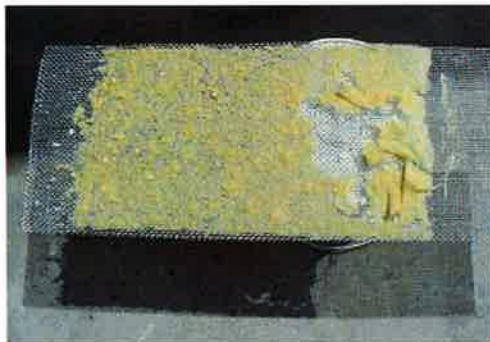
Screen of 1/8-in. Mesh Opening Obstructed by Cal-Sil (Small Yellow Lumps) and Fiberglass (Uniform Translucent Mat). Close Inspection Reveals Very Small to Microscopic Cal-Sil Granules Imbedded in a Complex Fiber Mat. The Broken Bed to the Right of the Photo Was Damaged During Screen Removal. Nominal Fiber Thickness is 1/10-in.
