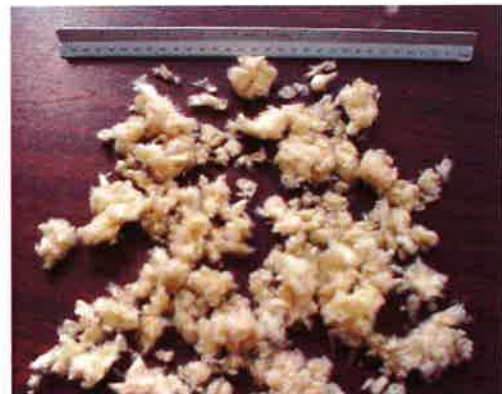
Typical Nukon fiberglass insulation debris used in transport testing.
